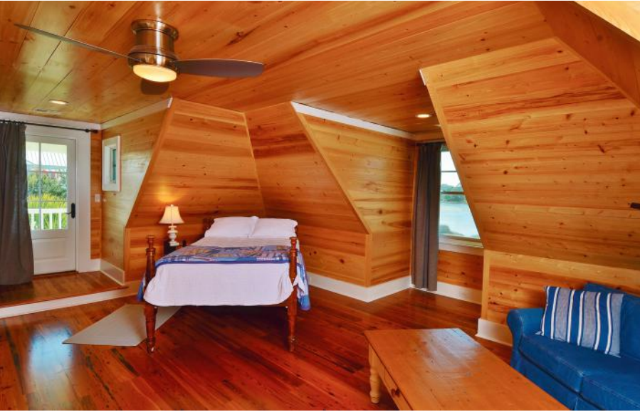
The upstairs bedroom of the home shown above was completely renovated by Calibre Development. Antique heart pine flooring, cypress walls & cypress ceilings were installed.
